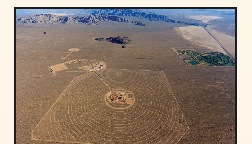
Left: Compact Linear Fresnel Reflector (CLFR) developed by Ausra now Areva Solar, photo 2009, courtesy of Ausra. Right: An aerial view of the first unit (120 MW) out of three (392 MW), of the BrightSource Energy Solar Electric Generating System, under construction at Ivanpah California, photo 2011, courtesy of BrightSource Energy.
